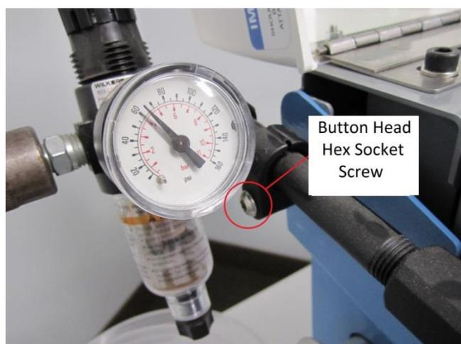
5. Remove the Left Side Lower Machine Cover from the Y151T-110/220 Machine
