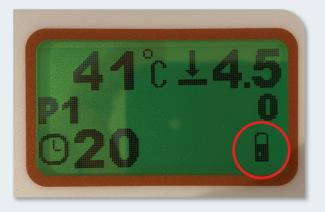
• Short press [AUTO] to release the machine. (photo 3: lock open)
