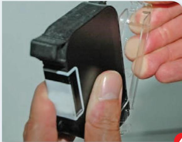
Gently lift the latch until the cartridge clip releases from the ink cartridge (see Figure 4)
