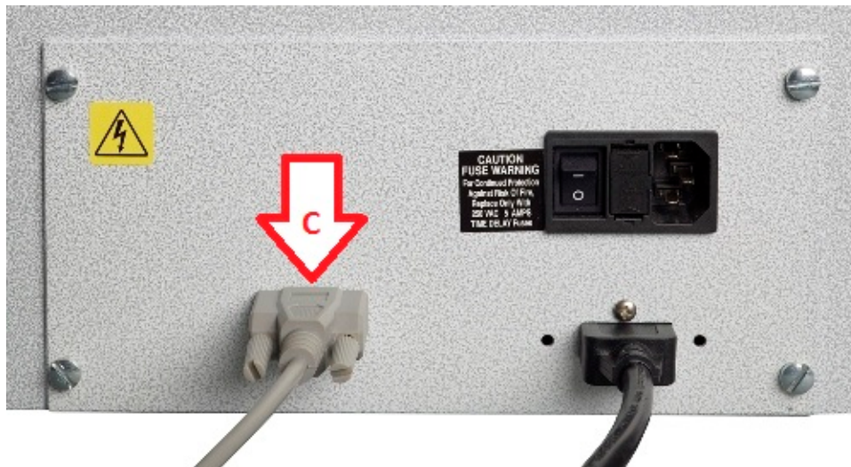
Figure 3 — Electrical Plugs Connected
